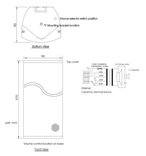
1. Remove the top cover of the unit (cable gland end) and connect the 100 volt line input cable into the ceramic terminal block through the cable gland provided.
